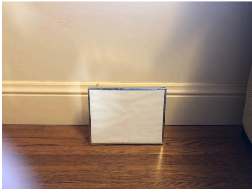
Figure 7. Panel in position to measure lower wall heat flow.
