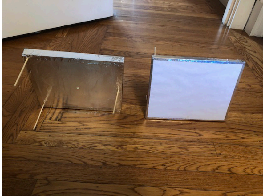
Figure 6: Panels used for measuring effective environment temperature.
